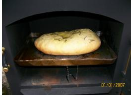
Note that the dry oven stove will reach higher cooking temperatures than the wet stove because of the cooling effect of the water heating boiler.
